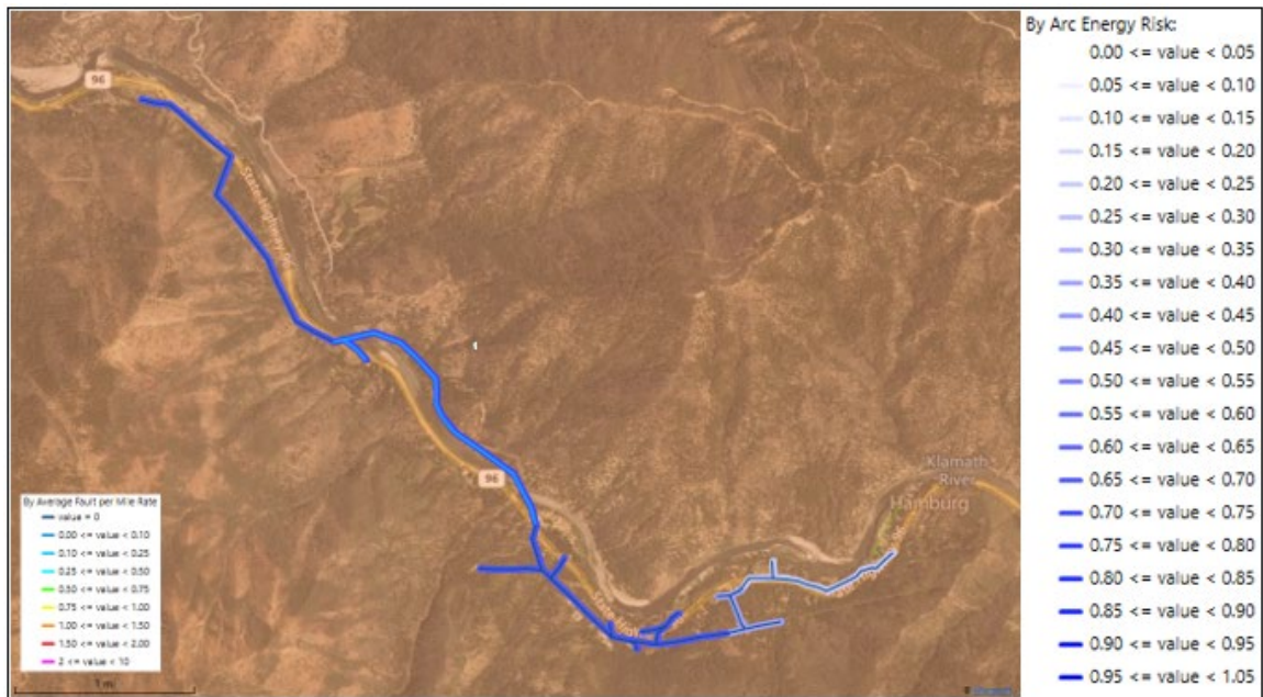
Figure 4.5-16: 8G27 with zonal Faults per Mile Rate overlaid with zonal Arc Energy score
