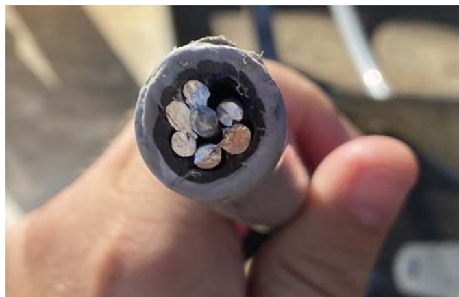
Figure 1 Three-Layered Covered Conductor
