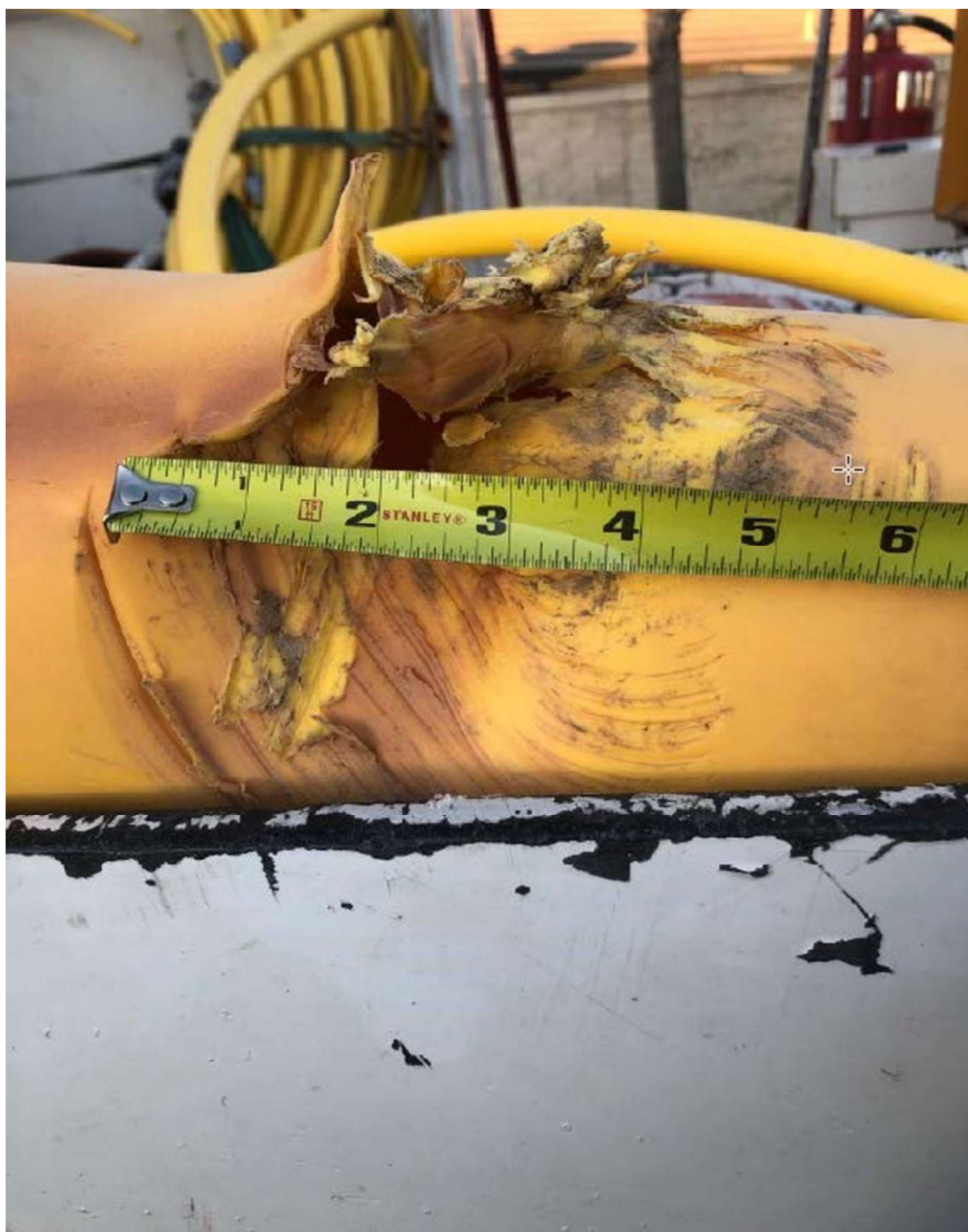
Photo 9: Damaged six-inch plastic gas main
