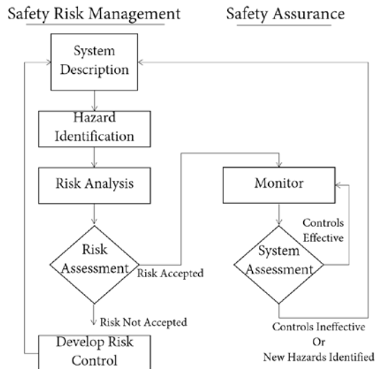
Figure 3: Modified Safety Risk Management/Safety Assurance Workflow. Simplified from Federal Aviation Administration Order 8040.4B: Safety Risk Management Policy, May 2, 2017, p. 9.
