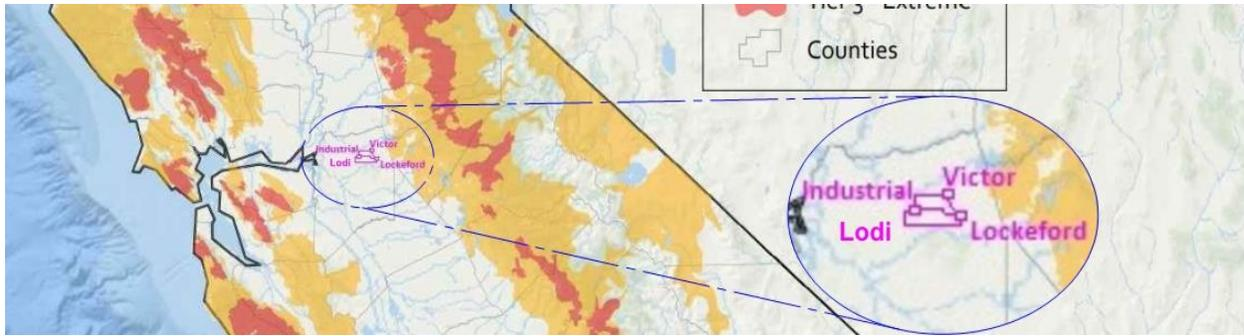
*Note: Three 60kV transmission lines originating from PG&E's Lockeford substation, operated and maintained by PG&E, enter LEU's service territory at the Industrial substation.*
