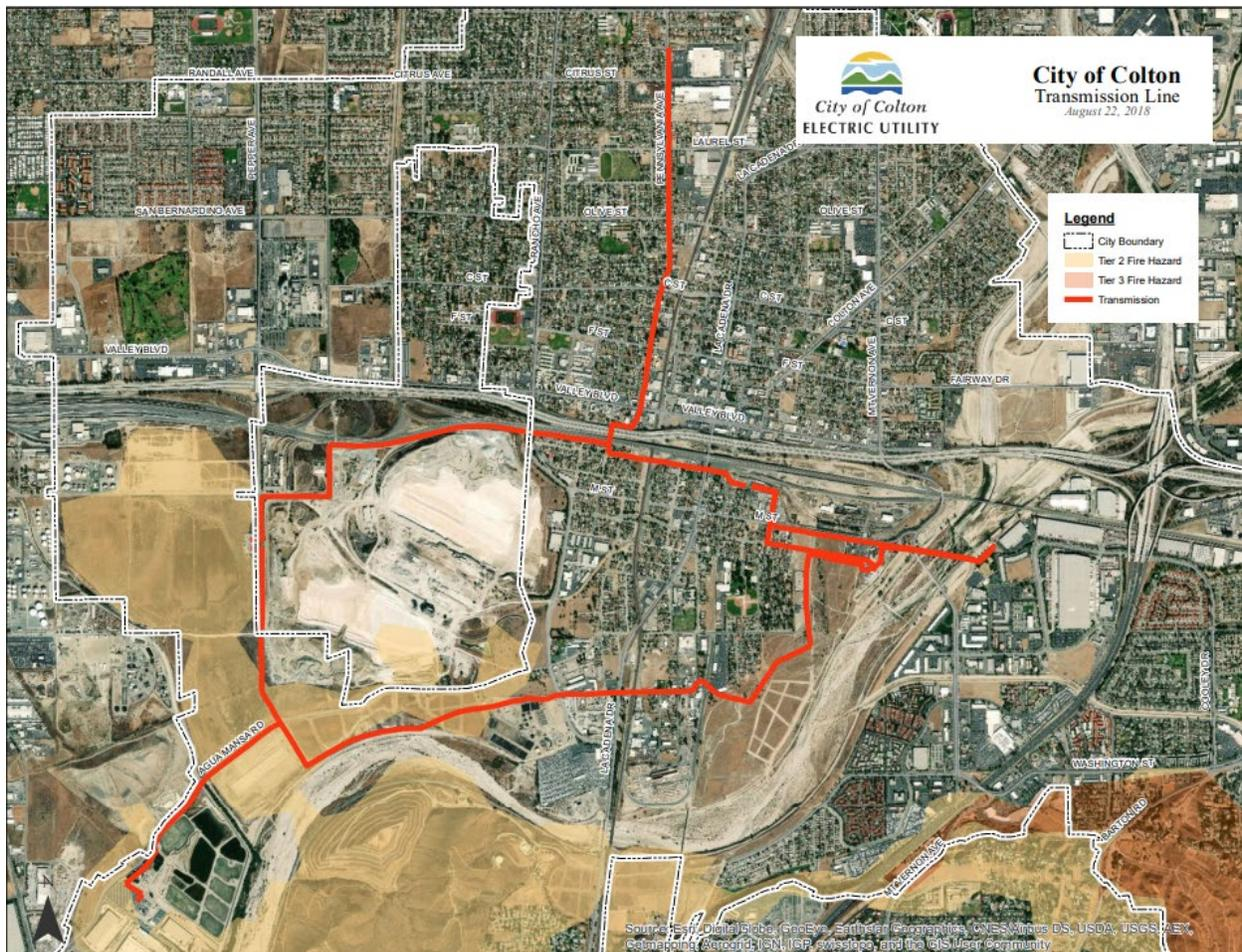
Figure 4: 66 kV Lines in Agua Mansa Industrial Corridor and Surrounding Area
