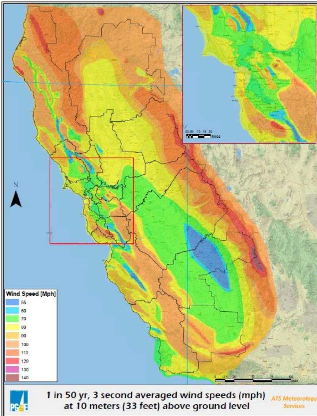
Figure 15 - PG&E 50 year return interval 3 second wind gust speed at 33 feet above the ground
