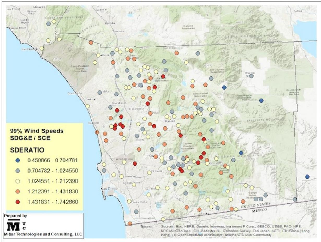
**Figure 11** - Ratio of SDG&E 99% wind gust station data to SCE 99% wind model.
