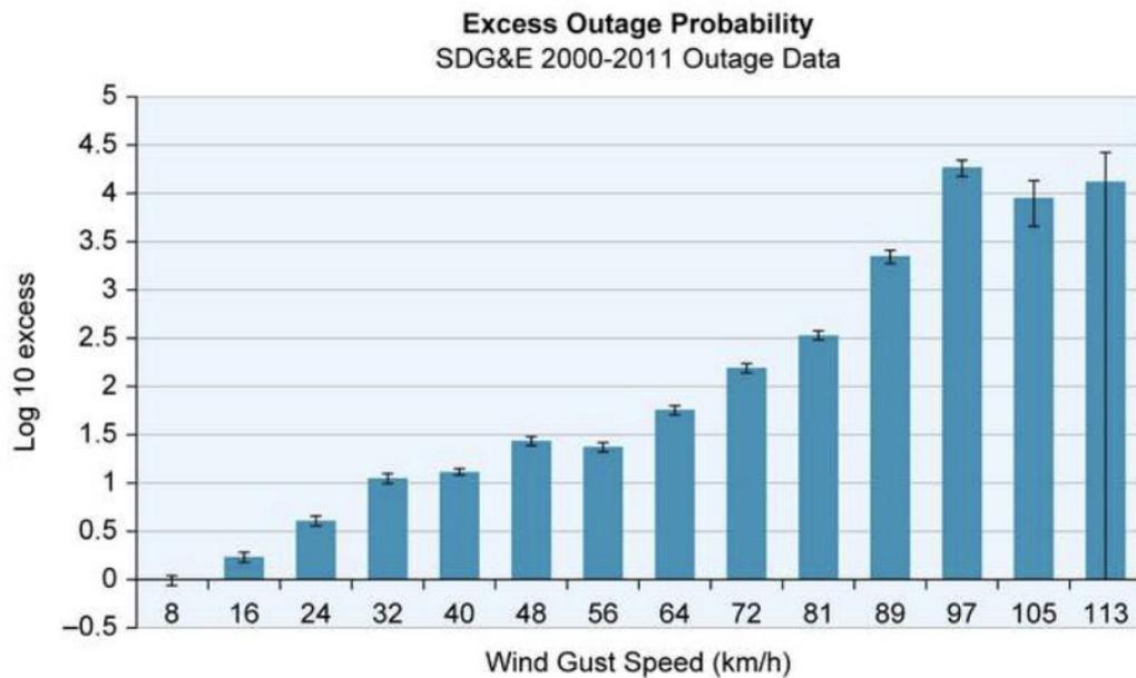
**Figure 1 - Outage rate as a function of wind speed<sup>18</sup>**
