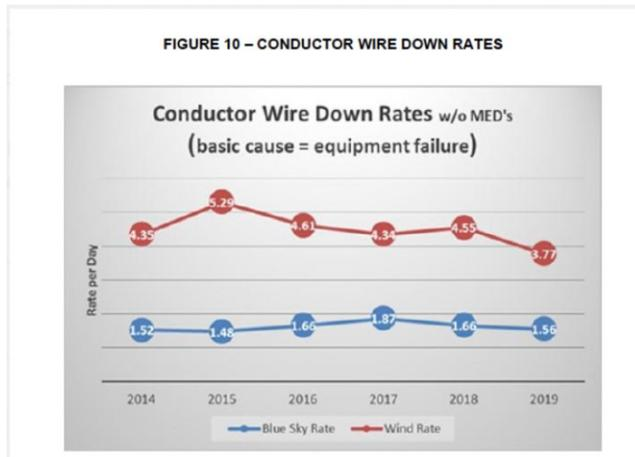
**Figure 2 - PG&E Conductor wire down rates due to equipment failure.**
