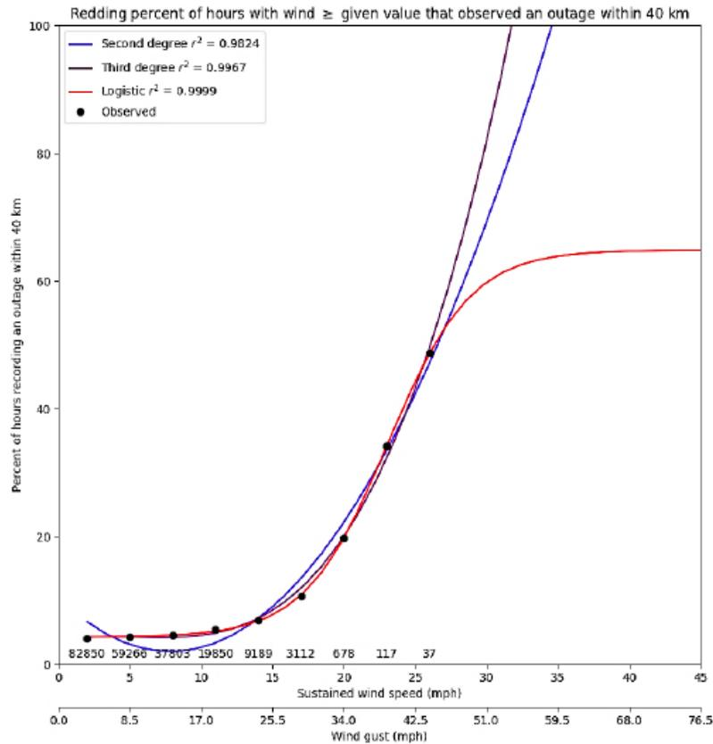
**Figure 1 - Figure 8 from PG&E Fire Risk document; p. 25, showing percentage of hours recording an outage within 40 km of Redding, CA as a function of sustained and continuous gust speeds.**
