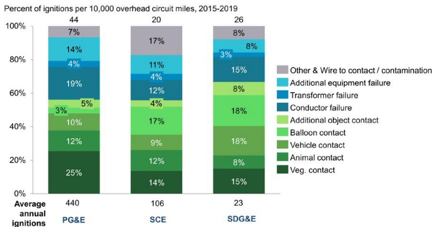
**Note: Conductor failure includes conductor failure (as reported), splice, clamp and connector. Other includes wire to wire contact / contamination.**
