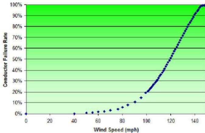
Figure 5-2. Florida Power & Light Span Failure Rate Data
