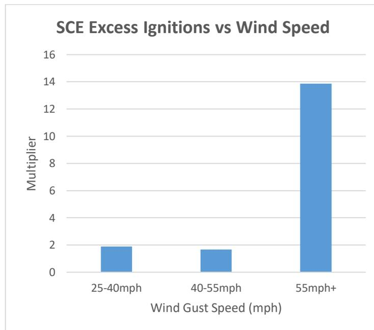
**Figure 8** - Excess ignitions above ambient wind speed for SCE 2015-2020 ignition data as compared against Monte Carlo data using the same ignition locations. The “multiplier” is determined by dividing measured ignitions by expected ignitions in each bin.
