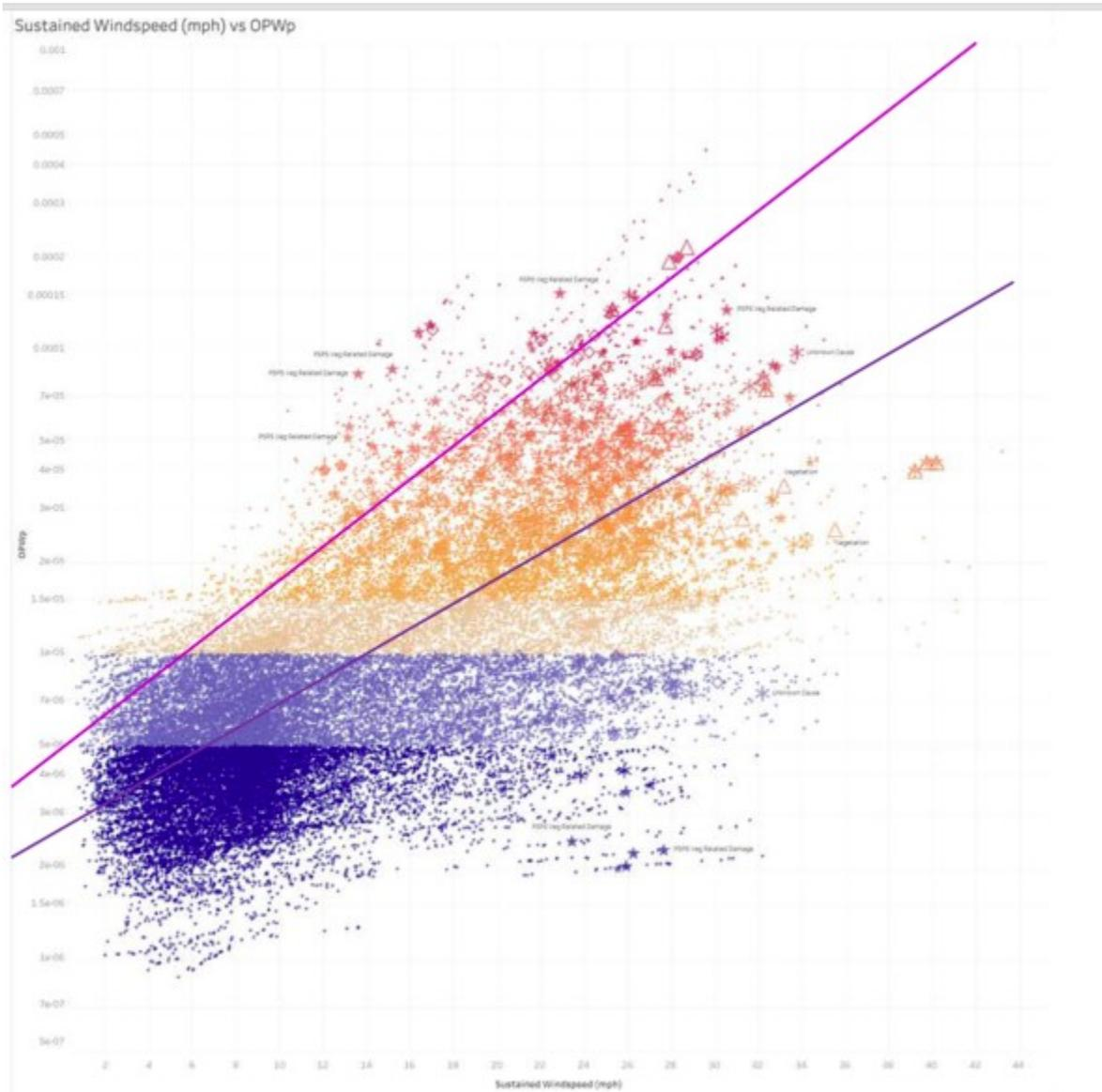
**Figure 7** - Excerpt from Figure PG&E-4.2-8 OPW Model. Lines have been added as guides to the eye (not a numerical fit), one showing "typical" wind dependency and one showing "high end" wind dependency. The "typical" dependency slope has a 0 mph intercept at  $3e-06$  and reaches a maximum of 0.00016 at 44 mph. The "high end" wind dependency has a 0 mph intercept at  $5e-06$  and reaches a maximum of .001 at 42 mph.
