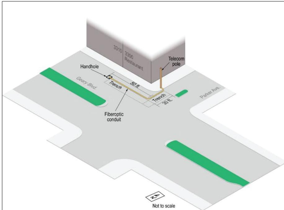
**Figure 3:** Excavation work plan for 2/6/19. Courtesy NTSB.
